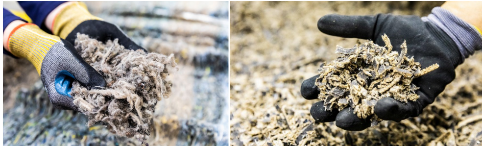
(Left): Fluff - high purity yarn (95%) - is generated by Tarkett's recycling center in Waalwijk, the Netherlands, before being sent to Aquafil. (Right): Shredded EcoBase backing separated from the carpet tile and recycled for the production of new EcoBase.
